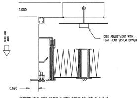
SECTION VIEW WITH FILTER SHOWN INSTALLED (SCALE 3/8:1)
